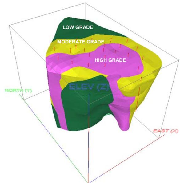
**Figure 6:** Macrodiamond sample grade distribution in Victor North PK (2001/2002 bulk sampling programme), courtesy of the Victor Project. Intervals on the vertical axis are 50m. Red markers indicate large diameter drillholes.
